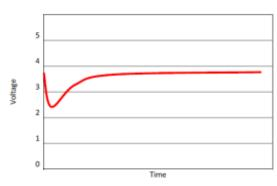
steady if other discharge conditions do not change. If the load increases after the cell's voltage stabilizes, then it may dip again until the passivation layer is sufficiently removed. Once the load is removed or lowered, the passivation layer will reform, and voltage delay may be a factor when subsequent loads are applied.
